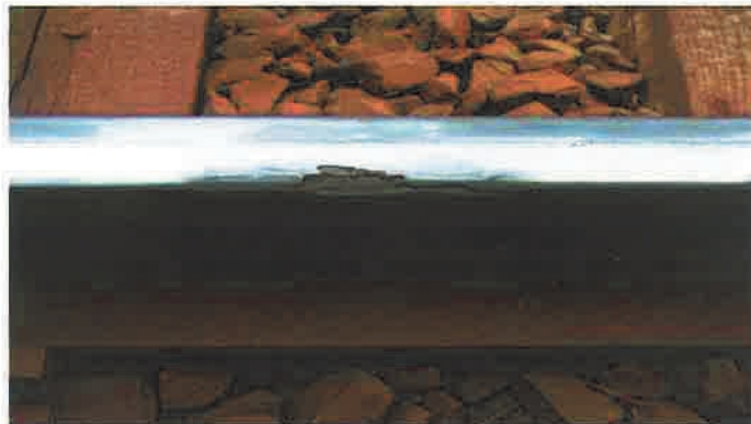
Example of shelling on the upper gauge corner.
