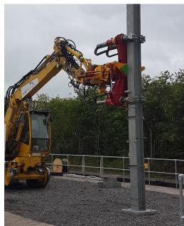
The Steel section Manipulator SM15 has been designed to handle, erect and install track electrification steel masts, for a safety use.
